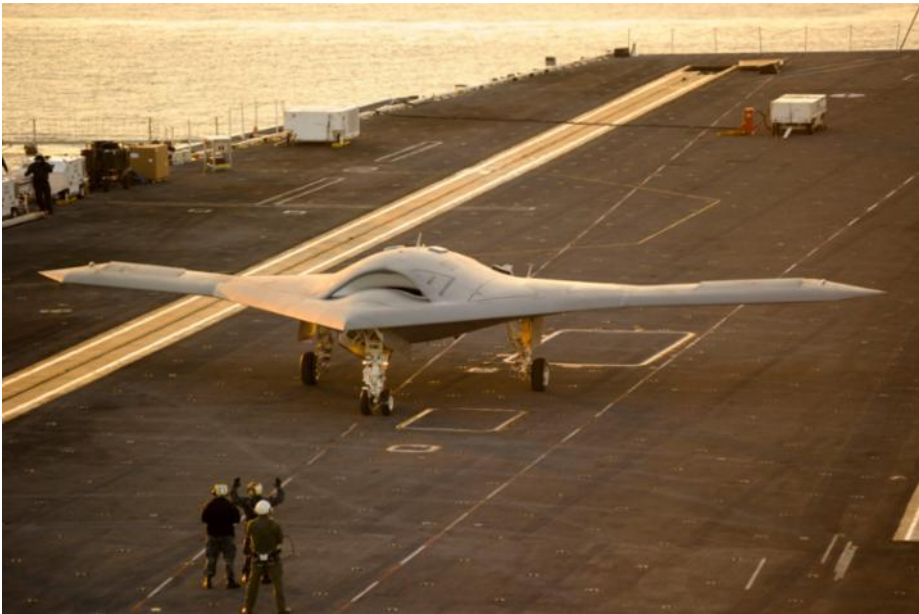
The X-47B Unmanned Combat Air Vehicle, developed by Northrop Grumman in cooperation with the US Defense Advanced Research Projects Agency, is semi-autonomous. (Courtesy of Northrop Grumman)
